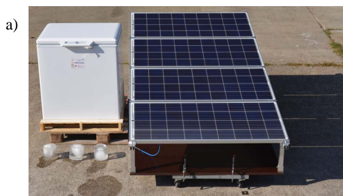
Figure 1. a) Solar Ice-maker connected to the solar panels y b) Insulated milk cans
