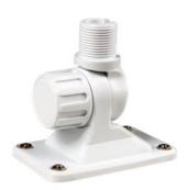
The lightweight SW2DK tilt-pivot swivel base made of high-strength nylon provides a firm grip through its four-point screw connection. With the handy turning device on the holder, the antenna can be quickly and easily tilted 2x 90 ° in both directions. The standardized 1 "x 14 BFS thread is compatible with our antennas. The cable guide on the thread allows the insertion of the cable even if a connector is already mounted on the cable.
