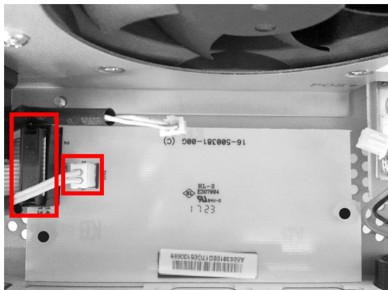
Figure 5: Remove connectors on beige dummy board
