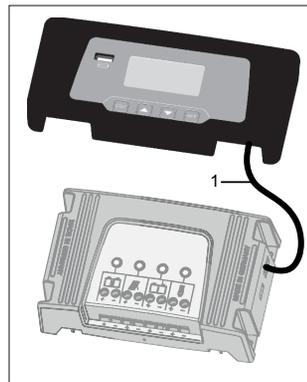
1. Insert the plug of the cable supplied (1) into the "StecaLink" connector of the remote display.
