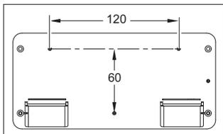
Dimensioned drawing for holes in casing base
