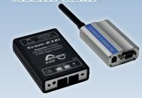
The set includes one Xcom-232i, one cellular modem and all necessary accessories. The SIM card is not provided.
