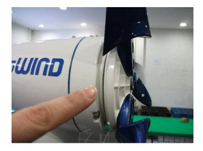
6. Attach the nose cone by pressing it against the hub
