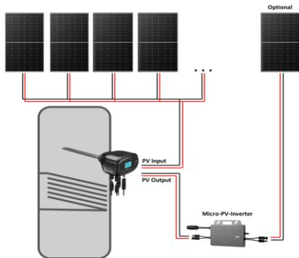
When the maximum temperature of the water in the hot water tank is reached, the switch can also be made to a micro PV inverter. This enables the efficient and bureaucracy-free surplus use of the generated solar power. In addition to hot water costs, electricity costs can also be reduced.
