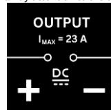
**IMPORTANT!** Do not connect any energy source to the output of the solar heating element! A return current into the solar heating element must be excluded. Always make sure that the polarity of the connected solar devices is correct. Failure to do so can lead to a defect in the solar heating element.
