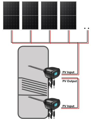
Two solar heating elements can be connected in series. This enables energy-efficient stratification of the hot water in the storage tank. As soon as the upper heating element has reached the maximum temperature, the switch to the second heating element takes place, which is located further down in the storage tank.
