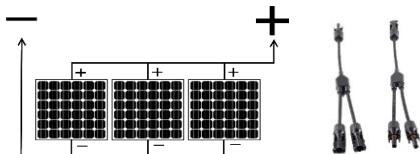
The photovoltaic modules are connected to the solar heating element to the solar input (see technical drawing: No. 5 Input – Input photovoltaic modules). The correct polarity of the photovoltaic modules to be connected can be found in the sticker on the solar heating element.
