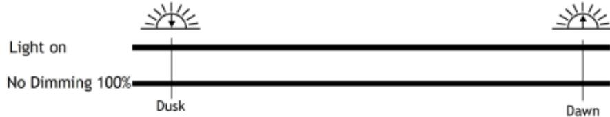
**NOTE:** Dimming can also be activated based on battery SOC/LVD. Set a value using rotary switch 10; if the battery voltage falls below the value, the dimming function is activated.
