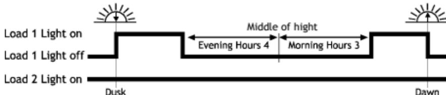
Night and day detection voltage (solar open circuit voltage):
